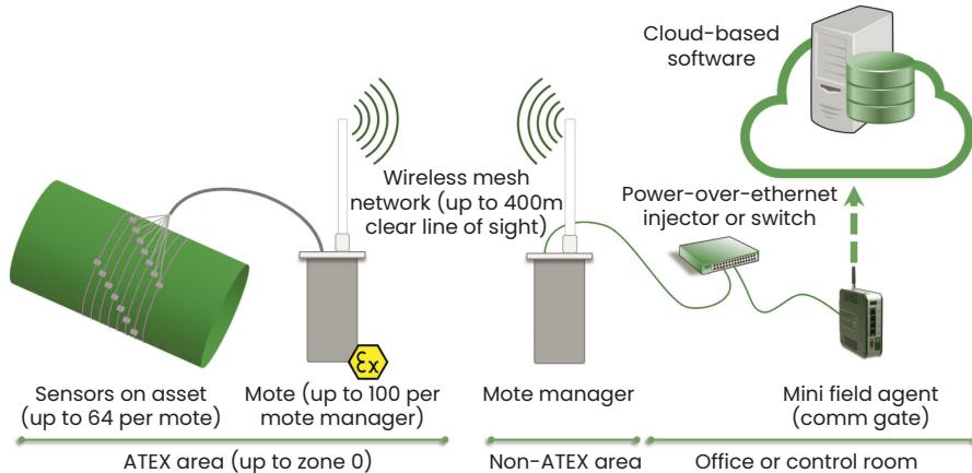
Figure 1 – Predictive Corrosion Management (PCM) elements
