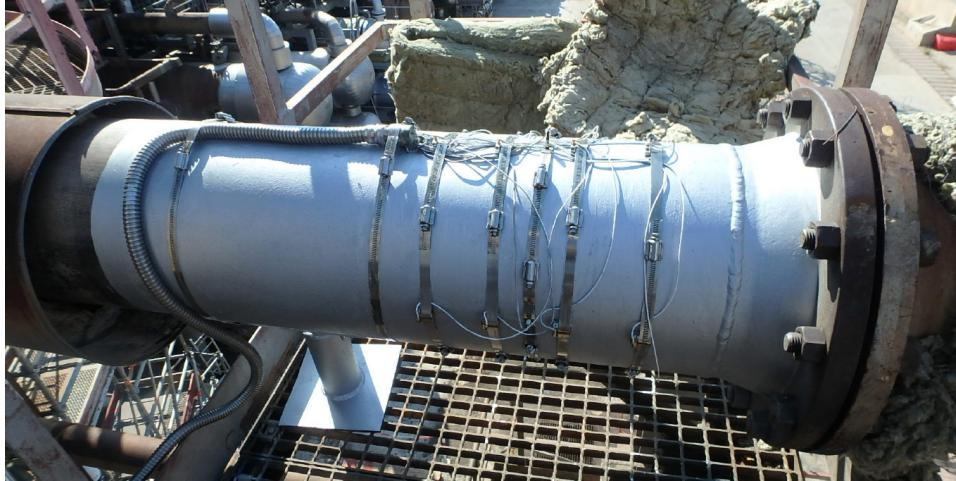
Photo 1 – Installation of UT sensors under insulation ( $T = 130^{\circ}\text{C} / 266^{\circ}\text{F}$ )
