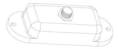
Figure 14: Conduit Cable Adapter, Single (Part Number 141887-01)
