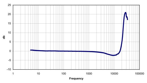
Figure 17: 200150 Amplitude Frequency Response (Typical)
