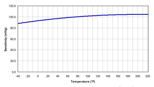
Figure 23: 20015x Accelerometer Temperature Sensitivity (Typical)
