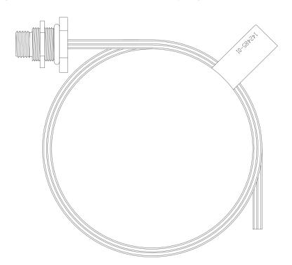
Figure 13: Housing Cable Adapter (Part Number 142485-01)
