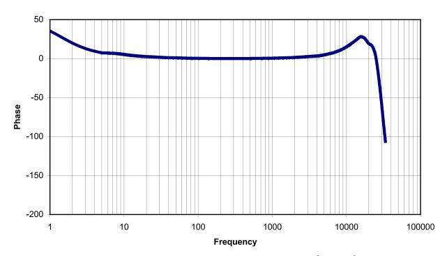
Figure 20: 200155 Phase Frequency Response (Typical)
