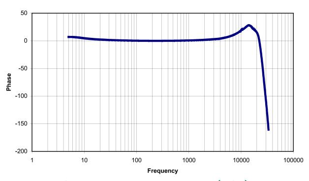
Figure 22: 200157 Phase Frequency Response (Typical)
