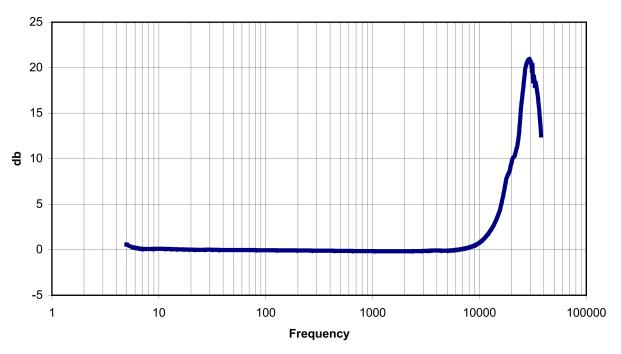
Figure 21: 200157 Amplitude Frequency Response (Typical)
