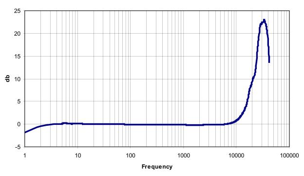
Figure 19: 200155 Amplitude Frequency Response (Typical)
