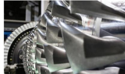
When a steam turbine exhibited sustained high vibration, concerned plant personnel consulted a Bently Nevada Machinery Diagnostics Engineer who remotely accessed the monitoring system, identified looseness in a bearing assembly, and confirmed that the unit could stay online, deferring repairs until a more convenient time. By conducting planned versus unplanned maintenance, \$900,000 USD of lost production was averted.
