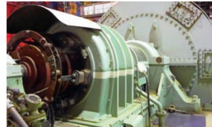
Using System 1 software and Bently Nevada machinery protection systems, a plant was able to diagnose shorted rotor bars on a generator, yet keep the unit online by balancing vibration levels and VARS to keep the thermal bow of the generator rotor to a minimum. VARS were shared across the other four units until this particular generator could be rewound during a planned outage. Since this is a baseload plant, the economic benefits accrued were substantial.
