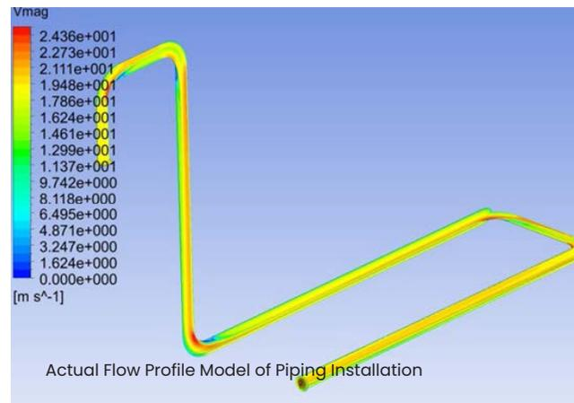
quantify pipe bend and other effects on flow profiles under a wide range of conditions. In most cases CFD analysis can accommodate pipe runs as short as 6 diameters upstream and 2 diameters downstream, with minimal effects on meter accuracy.
