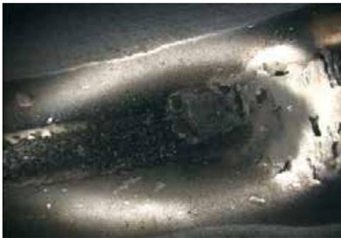
Bearing #1 - inner ring raceway showing severe wear path near the spalls
