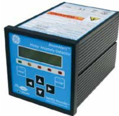
This system is applicable to 3-Ø AC, induction or synchronous, fixed or variable speed motors. AnomAlert provides both mechanical (unbalance, misalignment, and roller bearings, for instance) and electrical (loose windings, short circuits, etc.)
